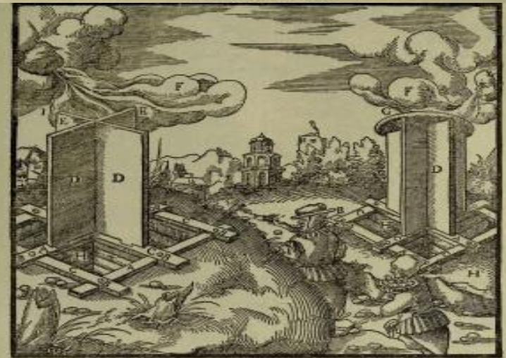
A—SILLS. B—POINTED STAKES. C—CROSS-BEAMS. D—UPRIGHT PLANKS. E—HOLLOWK. F—WINDS. G—COVERING DISC. H—SHAFTS. I—MACHINE WITHOUT A COVERING.
