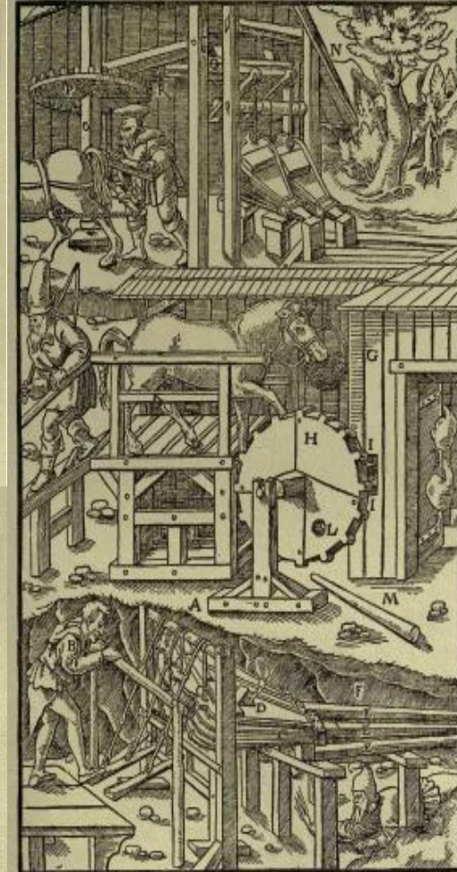
A—MACHINE FIRST DESCRIBED. B—THE WORKMAN, TREADING WITH HIS FEET, IS COMPRESSING THE BELLOWS. C—BELLOWS WITHOUT NOZZLES. D—HOLE BY WHICH HEAVY VAPOURS OR BLASTS ARE BLOWN OUT. E—CONDUIT. F—TUNNEL. G—SECOND MACHINE DESCRIBED. H—WOODEN WHEEL I—ITS STEPS. K—BARREL. L—HOLE IN SAME WHEEL. M—POLE. N—THIRD MACHINE DESCRIBED. O—UPRIGHT AXLE. P—ITS TOOTHED DRUM. Q—HORIZONTAL AXLE. R—ITS DRUM WHICH IS MADE OF HUNDLES.
